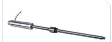
Linear actuators are more preferred for fin actuation systems in smart ammunition, guided missiles, etc., where volume and weight factors are exceedingly critical. FEMSAN manufactures linear actuators for precise guidance kit. For this, A ball screw or lead screw / nut assembly to slotless or coreless BLDC motor to translate the rotary motion to linear motion. In this regard, FEMSAN linear actuators are more precise motion source for fin actuation systems.
