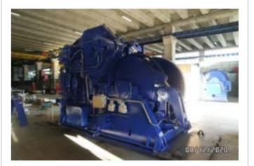
These will operate as part of the maneuvering equipment of the LCT ship. They will also be used in rope maneuvering via the warping end. For this purpose, there will be a drum and two warping end on the windlass.
