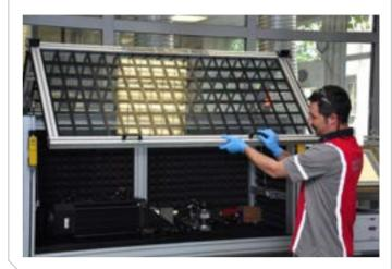
It is an aircraft engine washing system designed to perform periodic jet engine washing tasks defined by the manufacturers' CMMs for various types of jet engines.
