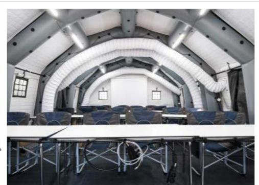
The tents have the features of quick installation, Waterproof, Flame retardant, UV resistance and snow and wind load resistance and they are used as Staff Tent, Command Post Tent, Warehouse Tent, Maintenance and Repair Tent, and Mobile Hospital.
