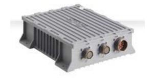
WIU (Weapon Interface Unit) is a 2 channel MIL-STD-1760D interface unit. It provides discrete and power signals required to manage and fire two weapon systems simultaneously. WIU increases system safety by monitoring and checking the validity of power and discrete signals. This feature decreases the possibility of inadvertent weapon firing. WIU provides the power and discrete signals in a redundant manner to increase total system reliability.
