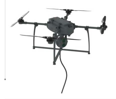
KIRLANGIC-X4C has the ability to perform its duties continuously due to its cable system and fixed power station. It meets the needs of reconnaissance, surveillance and intelligence in coastguard and border security control, security of critical facilities, disaster management and onscene security operations.
