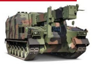
POYRAZ comes in as the support unit for FIRTINA T-155 Howitzer's ammunition supply where a vehicle's sustainability is a crucial aspect of its presence in the field. With a 96 units of ammo capacity, a POYRAZ can load 4 units of FIRTINA T-155 Howitzer during a single deployment.
