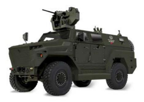
PUSAT Hybrid is being developed to meet the hybrid power system needs planned to be used in future combat conditions. The vehicle, which is being developed with series hybrid technology, charges the batteries by getting power from the Tümosan diesel engine. It can be used in battery mode with a range of up to 30 km according to different modes.
