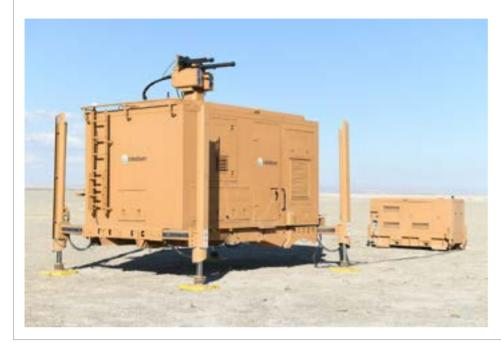
**ALKA Directed Energy** Weapon System [DEWS]; uses electromagnetic and laser technology against asymmetric threats as very close hybrid air defense system. Threats are interfered by Electromagnetic Jamming System [EJS] and are destroyed by Laser Destruction System [LDS] with two-layered defense architecture. It can also be used to counter bomb traps in residential areas and roadside Improvised Explosive Devices [IEDs].
