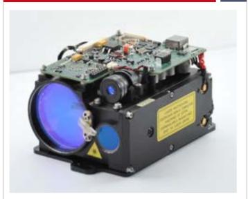
CETVEL-M10 is an eye-safe laser range finder to measure target distences for electro-optical sensor systems. Diode pumped laser source design enables the product perfectly matched with operational concepts of reconnaissance systems, targeting systems and electro-optical weapon systems.
