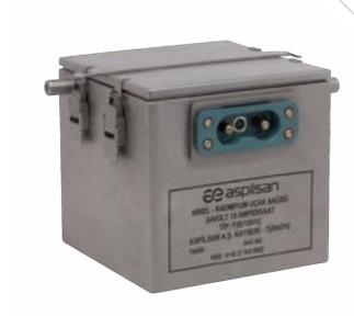
Battery is used in F-4, T-38,AB-206, NF-5, RF-5, CESSNA 210/310. It has a nominal voltage of 24 Volts, a nominal capacity of 15 Ah. It weighs 16.3 kg. The operating temperature range is -40 $^{\circ}$ C to +71 $^{\circ}$ C.
