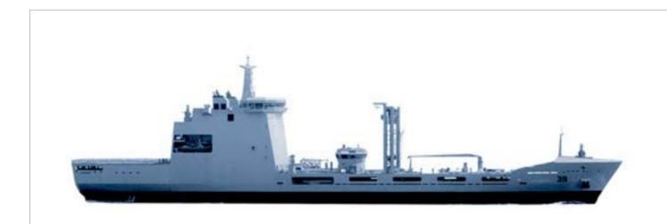
Logistics Support Ship is a double-hull vessel, designed for providing logistics support to the ships at sea in terms of dry and liquid cargo both during peace and war, equipped with conventional all dieasel-CPP propulsion system, conforming naval norms/standards and classification rules.
