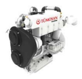
S8000 Marin is an engine with an engine volume of 3.9 liters, 4-cylinder in-line configuration, turbocharger aspiration and mechanical injection system. This engine, which can produce 105 HP at 2300 rpm, provides 350 Nm of torque at 1500 rpm. S8000 Marine is designed to provide powerful and stable performance in the marine industry.
