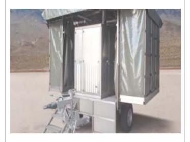
It is prepared for units that work in the field for short periods and frequently move. It consists of 9 compartment showers and the sections are separated from each other by a tarpaulin. 90 people can be washed in 90 minutes.
