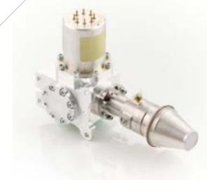
High performance MWIR detector developed for use in high-performance Electro-Optical Reconnaissance and Surveillance Systems designed by ASELSAN. FELIS-640/15-MW, integrated detector cooler assembly contains HgCdTe (Mercury Callium) active material, has 640x480 resolution and 15 µm pixel pitch, high operability, high responsivity, low read-out noise and programmable frame rate.
