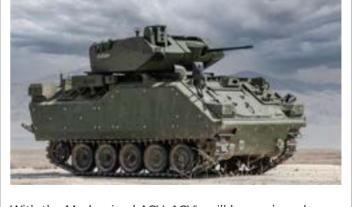
With the Modernized ACV, ACV's will be equipped with NEFER Unmanned Turret and high tech ASELSAN mission equipment like ORUMCEK 360° Close Situational Awareness System, Driver Vision System, Inertial Navigation System, Laser Warning System. Also Armor and Mine Protections are increased so that Modernized ACV's will have increased survivability and striking power on the battlefield.
