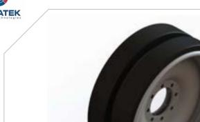
Road Wheels are other important components of running gear which create the interference between the support arm and the track assembly. They are basically metal rims vulcanized with a tough rubber around. Constantly working under high pressure and friction, the rubber's recipe and adhesion strength to the rim are key points to Road Wheel production.
