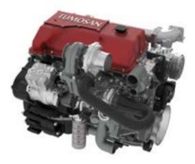
TMSN X5.5 is an industrial engine with a displacement of 5.2 liters and a 4-cylinder inline configuration. It is equipped with turbocharged aspiration and a common rail injection system. This engine can generate 232 kW of power at 2800 RPM and provides 1000 Nm of torque in the range of 1600-2100 RPM. With its low fuel consumption and high performance, it is a preferred choice for industrial applications.
