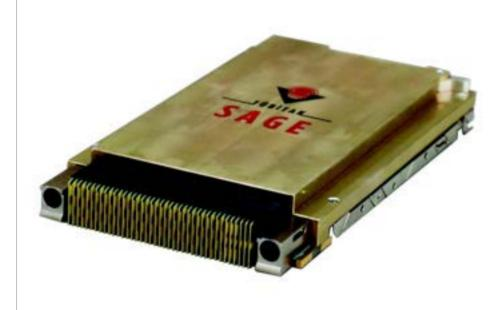
MKSK is compliant with OpenVPX (ANSI/VITA 65) 3U standards and designed by using System On Chip (SoC). It is designed for motor control requirements. Position data could be obtained as either digital or analog format. For digital position data, MKSK offers different kinds of digital interfaces.
