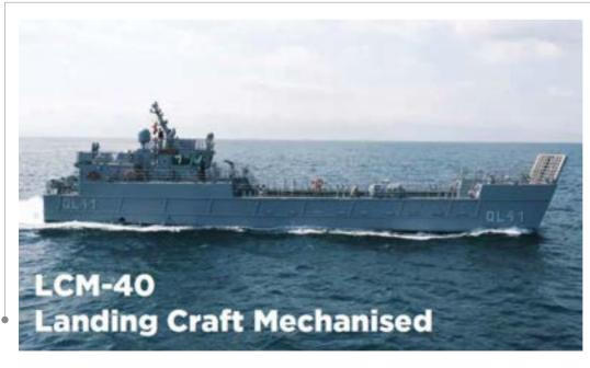
The LCM-40 is a Landing Craft Mechanized designed and built for transporting vehicles or troops ashore from the ship through the bow ramp by landing during amphibious operations. Additionally, in peacetime, they are used for personnel and vehicle transfers between military bases, ports, and various locations, including offshore platforms. 2 LCM-40s (QL41 ISHAT and QL40 BROOG) has been delievered to Qatar Navy.
