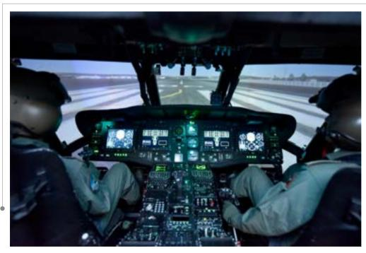
Rotary Wing Simulator is a turn-key integrated solution based on modern aviation school philosophy for the purpose of supporting the training of pilots and flight technicians. There are various synthetic training devices and supporting equipment such as Full and/or Partial Mission Simulators, Tactical Control Center, Computer-Based Training Rooms and Debriefing Systems, Training Management and Information Systems at the Training Centers.
