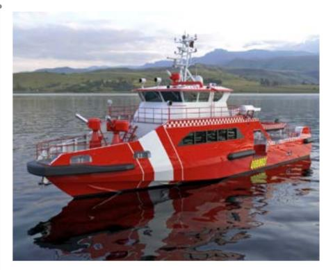
ARES 25 FiFi, the world's fastest fire-fighting vessel, is a well-proven design which is capable of fast intervention to fire incidents at sea such as oil & gas platforms, passenger cruise ships and inside & outside harbor incidents. As for construction material and classification rules the craft is very durable in terms of self fire resistance. The vessel has 2 fire monitors for incident response with a total capacity of 2400m<sup>3</sup>/h.
