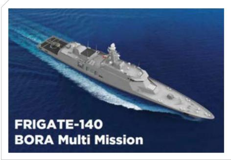
The 140-meter-long Frigate is designed to serve various purposes simultaneously. Equipped with its weapons and systems, its primary missions include ASuW, ASW, AAW, ISR, maritime security, border patrol, and helicopter operations. The vessel features two hangars for helicopter and unmanned aerial vehicle (UAV) operations. This versatile platform is capable of fulfilling various roles in naval operations.
