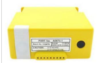
The battery is used in Emergency Locator Transmitter (ELT). It has a nominal voltage of 12 Volts and a nominal capacity of 300mAh. The maximum discharge current is 2.5 A. The operating temperature range is -60°C to +70°C.
