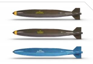
500 lb. MK 82 GP AIRCRAFT BOMBs have three variants. MK82 MOD1 HE is 239 g, is 2268±11 mm long, has TNT as filler and the filler weight is 87 kg. As fuze, it has M904 (Nose Fuze) and M905 (Tail Fuze). MK82 MOD1 PRE-FRAGMENTED is 245 g, is 2280 mm long, has TNT as filler and the filler weight is 46 kg. As fuze, it has AB 104 LAPT980. MK82 MOD1 PRACTICE is 234 g, is 2268±11 mm long, has Sorel Cement as filler. It uses a Dummy fuze.
