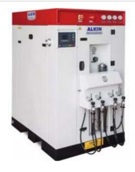
W4 series compressors have proven themselves in industries compressed air and breathing air are required for many years, thanks to their strong and powerful design. The user-friendly PLC-based control panel efficiently meets your compressor management, data tracking, help, and communication needs. It is a 4-stage reciprocating compressor with splash lubrication in its soundproof cabin. Compressed air capacity ranges from 500 to 1000 liters per minute at a maximum working pressure of 415 bar.
