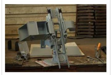
It is a platform produced for the connection of the heavy machine gun used on the ship to the deck.
