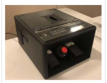
Engine Turning Tool (ETT) is used in borescope inspection operations on aircraft engines. It is designed to facilitate position control of turbine stages using servo motor and operator panel.
