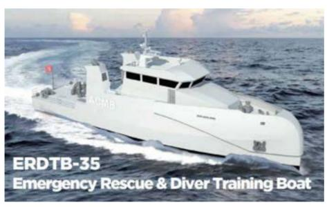
The ERDTB-35 is a Emergency Rescue and Diver Training Boat designed for providing diving training to trainees, conducting emergency interventions, and performing diving operations. It includes a decompression chamber for treating decompression sickness and is equipped with an underwater telephone system to support submarine rescue operations.
