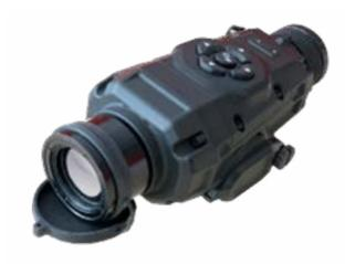
ATAY-200 is a STINGER MANPADS sight. Device has an infrared imaging technology with 640x480, 17µ resolution micro bolometer detector operating in the 8-12 µm band.
