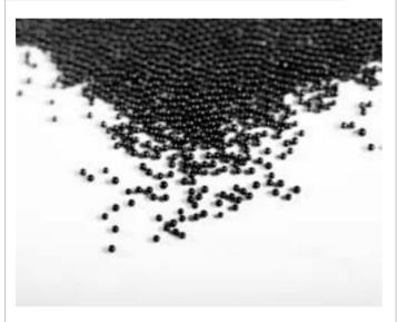
Our spherical activated carbons with high surface area and large pore structure are used in CBRN protective suits and systems that require special filtration.
