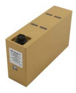
The rated capacity of the lithium-ion battery with a nominal voltage of 28.8V, which meets civil and military standards, is  $2 \times 10.3$  Ah. The charge temperature range of the battery is  $0^{\circ}\text{C}$  - +45°C; The storage temperature is  $20^{\circ}\text{C}$  (1 year) / -5 to  $25^{\circ}\text{C}$  (1 and 3 months).
