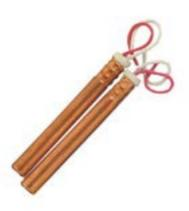
It is a detonator which has electrically ignitable fusehead by the action of dynamo type or condenser type exploder. It is used to explode the permitted explo-sives in the gassy and dusty mines (coal mines etc.) Tube material is copper and the deto-nator is firedamp safe. It can be manufactured at the desired cable length.
