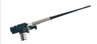
Is 113+8 kg, 2630 mm long and has 1500 m effective range with 125-400 rounds/ min rate of fire. It has double feeding with a 3 min time for ammunitions.
