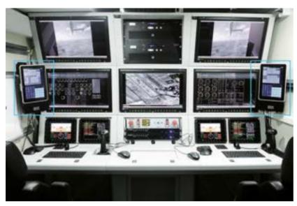
It's flexible, reliable, and efficient voice communication solution designed specifically for UAV. Based on Voice over Internet Protocol (VoIP) technologies, it enables the effective integration of multiple communication devices, including HF/VHF/UHF radios (digital or analog), various telephone interfaces, SATCOM, GSM, intercom systems, and legacy audio distribution systems.
