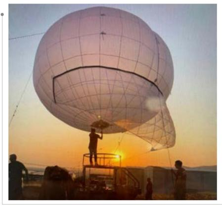
Surveillance Balloon is a mobile aerostat system inflated by helium. It allows day and night observation/surveillance operations at 300-500 m altitude. It can perform a wide range of missions such as homeland security, border security, traffic control and environmental surveillance, and also wildfire early warning.
