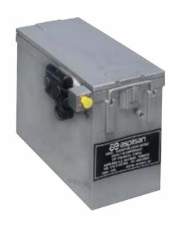
The battery is used in COUGAR AS-532 and SUPER PUMA. It has a nominal voltage of 24 Volts, a nominal capacity of 40 Ah. It weighs 38 kg. The operating temperature range is -40 $^{\circ}$ C to +71 $^{\circ}$ C.
