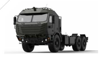
SEYİT 6x6 Tactical Wheeled Vehicle can climb up to 60% slopes and move on 30% side-sloped terrain while providing a maximum level of personnel safety with the high ballistic and mine protection level. SEYİT 6x6 has 16 tons payload capacity and high payload carrying area. SEYİT 6x6 can carry the heaviest systems without compromising vehicle performance.
