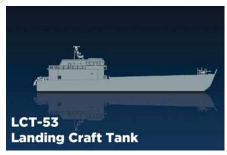
The LCT-53 is an Landing Craft Tank designed for transporting vehicles or troops ashore through the bow ramp by landing during amphibious operations. Additionally, in peacetime, it provides support for humanitarian aid and evacuation/rescue operations.
