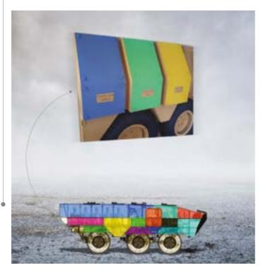
Multi-layered ballistic protection add-on armor solutions are optimized for keeping minumum effect on power to weight ratio change on platform. Add-on armor solution has capability to withstand both KE and IED threats.
