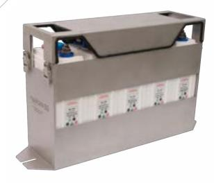
There are two different versions. The first one has a nominal voltage of 24 volts and a nominal capacity of 40Ah. It contains 20 cells in the FP40H1C-D cell type. The second has a nominal voltage of 6 volts and a nominal capacity of 145 Ah. It contains 5 cells in the KRX 145p cell type.
