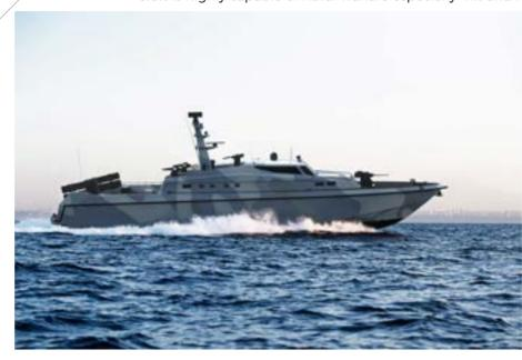
and infrared signature. The craft is equipped with auto-stabilized remote-controlled naval weapon systems to provide versatile firepower that can be adapted to a wide variety of potential scenarios. The vessel has a suite of naval communications equipment, combat management system, electro-optic (E/O) sensors and 2D Naval Radar. The vessel can launch and recover a military type RHIB for boarding and SAR missions.
