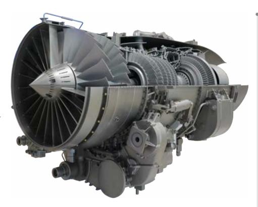
TEI-TJ30 is a micro turbojet engine that produces 125 Newton thrust with a diameter of 108 mm and a weight of 1.45 kilograms and can be used for different purposes such as missiles, target aircraft, RC aircraft and sports aviation. The engine can run on Jet A1, diesel, kerosene, JP8 or JP10 fuels.
