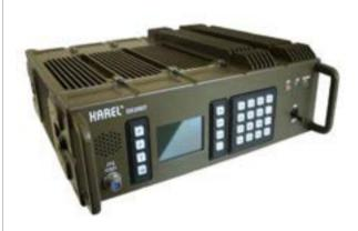
DS200T is a tactical IP communication system for military applications. DS200T is designed for field use and shock/waterproof. the system provides IP/SIP facilities for the military operations with its combat net radio connection capability. DS200T supports Co/PSTN lines, analog subscribers, E&M and ISDN PRI/E1 interfaces.
