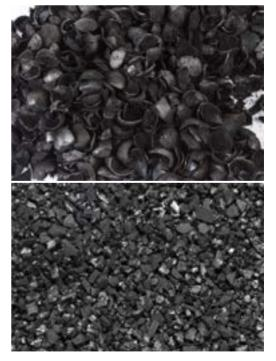
Granular, pellet and powder activated carbons are used in all kinds of filter systems.
