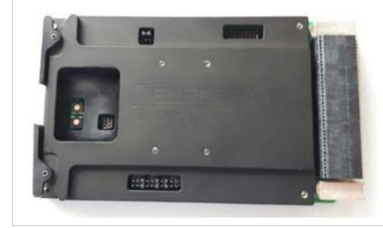
The BitFlex-VPX3-MZQ1 is a high-performance FPGA processing module based on the Xilinx Zynq family of FPGAs. It provides multiple high-speed fabric interfaces, external memory, an FMC site, and high-density I/O. It is ideal for customizable, high-bandwidth, signal-processing and image-processing applications.
