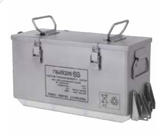
Battery is used in MI-17 and MI-18. It has a nominal voltage of 24 Volts, a nominal capacity of 27 Ah. It weighs 29 kg. The operating temperature range is -40°C to +71°C.
