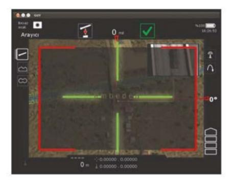
Fire Control Unit is the electronic work package of the System, and has two different modes: tactical mode and simulation mode. Since it can simulate all control operations in tactical mode for training purposes, it allows the user to train without the need for an external device.
