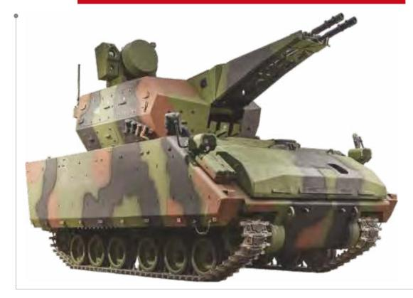
Is 432 kg in total, is 4.424 mm long with barrel and muzzle brake and has 4000 m effective range with 2x550 round/ min rate of fire.
