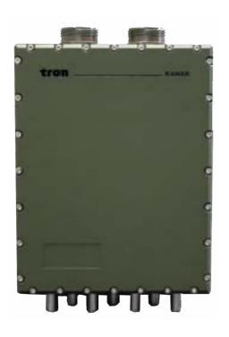
The TRDF-3000-7-14 is a switchable antenna switching unit housed in a single-block aluminum enclosure, featuring isolated RF boards. Operating within a frequency range of 20-3000 MHz, this unit is equipped with 14 RF inputs and 7 RF outputs, and is designed to withstand high input power levels. It offers operational flexibility with remote control via TTL and RS422 interfaces. With its robust and reliable performance, this switching unit is the right choice for professional RF applications.
