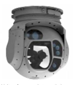
CATS is a high-performance electro-optical, reconnaissance, surveillance and targeting system developed for Unmanned Aerial Vehicles (UAV). Multispectral (MWIR, HD Day TV, LL-NIR) optical aperture combines multiple optical channels in a single channel so that the system has high range and imaging performance even in adverse weather conditions without increasing size and weight.
