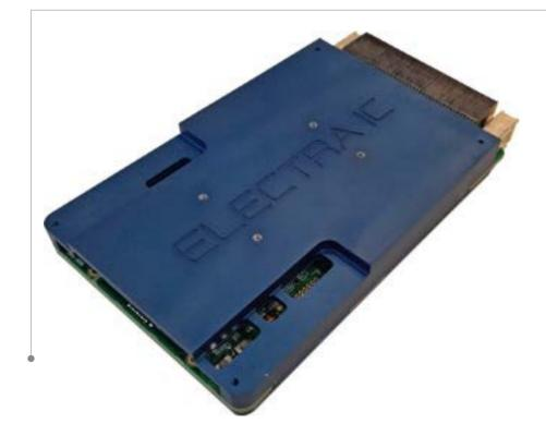
The BitFlex-VPX3-MZQU is a high-performance FPGA processing module based on the Xilinx Zynq UltraScale + family of FPGAs. It provides multiple high-speed fabric interfaces, external memory, an FMC site and high-density I/O. It is ideal for customizable, high-bandwidth, signal-processing and image-processing applications.
