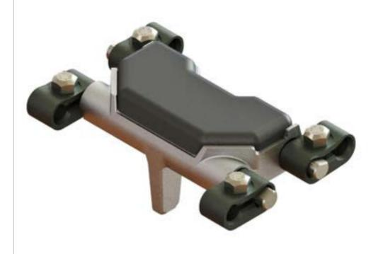
Track Assembly is a unique component which provides the vehicle mobility. By transmitting the torque coming from the final drive into directional movement, it enables the tracked platforms to move in almost all types of terrain. Track assembly composes of center guide, track shoe links and each links are connected with end connectors.
