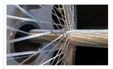
It is a shielding product known as Conduit. Stainless steel spiral hose used as steel body is a general purpose high quality connection hose. It is made of AISI 304L Stainless Steel material. Tin plated copper wire braided on steel body. It is produced in 10 different diameters from 10.7 mm to 62.4 mm.
