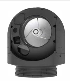
ASELFLIR-500 is a high performance electro-optical Technical Specifications reconnaissance, surveillance and targeting system developed for fixed-wing and rotary-wing aerial platforms including Unmanned Aerial Vehicles (UAV), Helicopters and Airplanes. ASELFLIR-500 system includes 3-5 micrometer High Resolution Infrared Camera, High Resolution Day TV Camera, High Resolution SWIR Camera, Laser Target Designator, Laser Range Finder, Laser Spot Tracker and Laser Pointing units.
