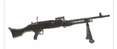
Has Open Bolt. Accuracy is 8 MOA, it is M13 Belt feed from left and is 12 000 g. Effective range is 800 m and has 650-950 rds/min fire rate. It is Full-automatic.
