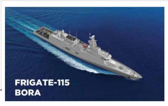
The 115-meter-long Frigate is designed to serve various purposes simultaneously. Equipped with its weapons and systems, its primary missions include ASuW, ASW, AAW, ISR, maritime security, border patrol, and helicopter operations. The vessel features two hangars for helicopter and unmanned aerial vehicle (UAV) operations. This versatile platform is capable of fulfilling various roles in naval operations.
