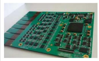
FPGA based structure offers re-programmable messaging structure. 5 Mbps serial interface to control RF modules via various messages scenarios. Supervisory circuit provides overvoltage protection for RF modules.
