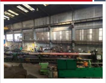
It is a very important transmission organ that transfers the rotational motion it receives from the engine to the propeller. They are made entirely of stainless steel or forged steel. These shafts, which come in different lengths and diameters, are long cylindrical rods (shafts) as we know them.
