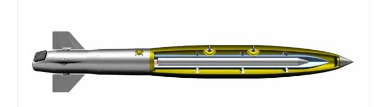
SERT-82 has identical external geometry, guidance unit interfaces, mass, center of mass and intertia properties with Mk-82 GPB.
