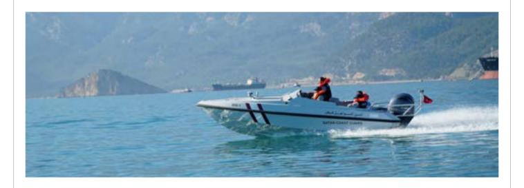
ARES 25 CAT FiFi is a proven design by BMT developed for maritime fire-fighting, search and rescue operations. As for construction material and classification rules the craft is very durable in terms of self fire resistance. The vessel has 2 fire monitors for incident response with a total capacity of 2400m<sup>3</sup>/h.
