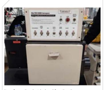
It performs the electrical and functional tests of the smoke detectors used in the aircraft cabin and cargo compartments.
