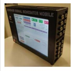
It is a multi-channel portable signal generator and encodes all ARINC429 labels and adds functionality to them.
