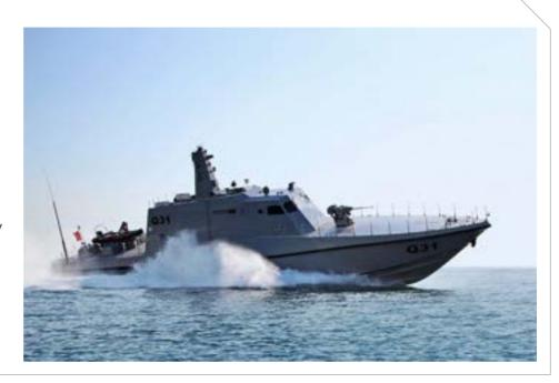
Mrtp12 fast patrol boat (sdb) has been specially designed for the Turkish Navy for the protection of highvalue units in bases and ports. It is equipped with 12.7 mm stabilized turret. The wheelhouse is ballistic protected. With 2 diesel engines and water jet propulsion system, the speed can reach up to 45kts. There are currently 8 of them in the inventory of the Turkish Navy. Length: 12,65m, width: 3,45m
