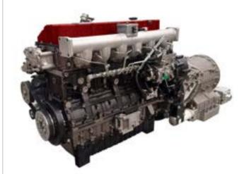
Power pack consisting of TMSN X 7.5 model engine and TMSN 2506 AT model transmission, with 7.8 lt engine volume and 530 HP Rated Power at 2400 rpm.
