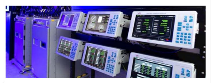
HAVELSAN Ship Data Distribution System (GVDS), a member of the HAVELSAN Platform Data Distribution Systems (PVDS) family, is designed to operate with full performance under any environmental condition of surface platforms. HAVELSAN GVDS, a redundant and reliable system, is developed for use on large, medium and small-sized warships with its 24/7 warfighting readiness and is a key system for the integration of ship systems.
