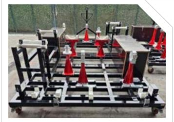
When the landing gear of aircraft coming for maintenance needs to be replaced, transportation and protection of the removed component poses a problem since there is no dolly for the removed landing gear.
