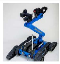
Suitable for remote tactical mobile applications in combination with a pluggable 6-axis manipulator arm and remote control console, which can be carried by a single user or two users.
