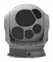
DENİZGÖZÜ-PİRANA is an electro-optical reconnaissance, surveillance and targeting system which operates in day and night and under all environmental conditions. DENİZGÖZÜ-PİRANA has MWIR Thermal Camera, SWIR Thermal Camera, Day TV Camera, Laser Target Designator, Laser Range Finder and covers 360° in azimuth. DENİZGÖZÜ-PİRANA can be integrated to Unmanned Surface Vehicles, Armed Unmanned Surface Vehicles, Boats, Corvettes according to platform requirements.
