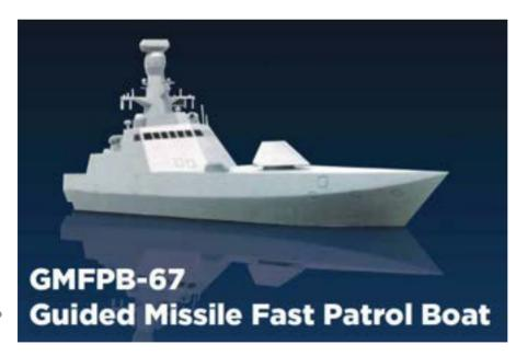
The GMFPB-67 is a Guided Missile Fast Patrol Boat designed primarily for conducting ASuW, ISR, and patrol duties, up to Sea State 5 conditions. Equipped with a wide range of weapons and systems, extensive radar coverage, and a high speed of up to 55 knots, it can efficiently perform patrol tasks and, when required, carry out search and rescue operations even in nighttime and limited visibility conditions.
