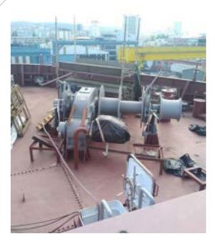
Anchor windlasses will work as part of the anchoring equipment and can also be used in rope maneuvering via their warping end.
