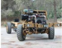
10 TONS MULTIPURPOSE ROLLING CHASSIS PLATFORM
