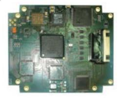
VideoDecoding/Encoding Unit comprises two parts. First unit compresses the digital video data received from the onboard imaging source of the missile by using the JPEG 2000 algorithm, and transmits it to the Video Decoding Unit (VDU) via the RS485 UART data bus through a data link or the central link. The second part is the VDU. This unit processes the data sent by the VEU and provides a video image.
