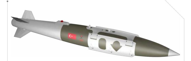
HGK-83 is a GPS/INS guidance kit that turns existing 1000 lb Mk-83 general purpose bombs into air to ground smart weapons which can be released multiple by using BRU 57 ejector rack.
