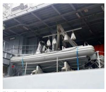
This will work as a part of the ship and can be used for launching and retrieving the boat from the sea.
