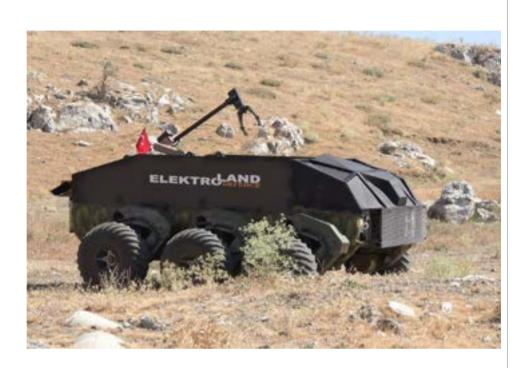
It is specially designed to neutralize traps such as ditches, barricades, culverts and bombladen vehicles from a distance.
