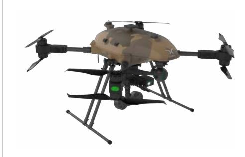
FALCON-SIHA is a Rotary-Wing Armed UAV system that stands out with its 2-axis stabilized motion capability, 5.56 mm caliber infantry rifle, superior recoil dampening system, and high ammunition carrying capacity. It is designed to directly hit the target with high accuracy or suppress the target with single or burst fire modes, depending on the mission scenario.
