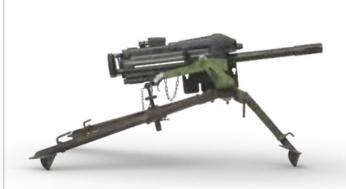
Is 62,5 kg in total, 1097 mm long, has a maximum effective range of 1500 m with rate of fires 325-375 rds/min for cyclic, 60 rds/min for rapid and 40 rds/min for sustained. It has 24 grooves and uses HE, HEDP, TP type bullets.
