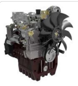
It is a member of the S8000 engine family, with a volume of 3.9 liters, in-line 4-cylinder, mechanical injection. It features turbocharged aspiration and provides 115 HP nominal power at 2300 RPM and 530 Nm of torque at 1500 RPM. This engine, which has a Stage 3A emission certificate, is environmentally friendly. Designed for industrial and generator applications, the S8000 offers users a stable and efficient operating experience.
