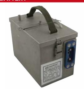
The battery is used in the F-16(BLOCK 40-50). It has a nominal voltage of 24 Volts, a nominal capacity of 17 Ah. It weighs 19 kg. The operating temperature range is  $-40^{\circ}$ C to  $+70^{\circ}$ C.
