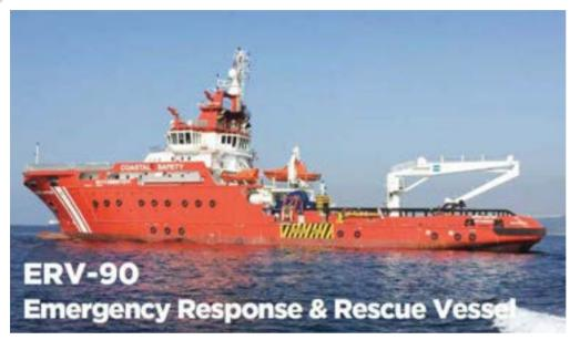
The ERV-90 is a Emergency Response and Rescue Vessel designed and built for various purposes, including ship recovery, salvage and towage with a 200 tons bollard pull capacity, firefighting, oil pollution prevention, and serving as a diving platform vessel. It also features a helipad for helicopter operations.
