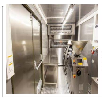
The oven has the capacity to bake 6240 pieces (150 gr) of bread in 8 hours. The oven unit consists of three 20 foot containers: preparation, baking and proofing containers. The inside of the containers are covered with stainless steel. A diesel generator is available for power outages. It has a capacity of at least 2000 liters that can be carried with the container. There is one main and one spare clean water tank.
