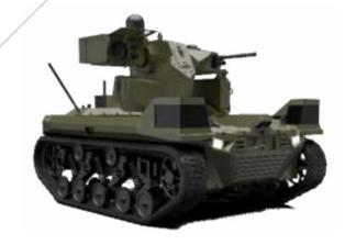
ASLAN is an Unmanned Ground Vehicle with high mobility that can be controlled autonomously or remotely, which can be used for reconnaissance, surveillance and on which the Laser Guided Mini Missile System, SARP-L weapon system, Tethered Drone System and Long-Range Acoustic System or other required systems can be mounted.
