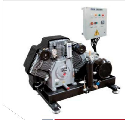
Compressors in the medium pressure series deliver compressed air up to 80 bar safely and effectively. These compressors have two-staged, reciprocating, air-cooled, splash lubricated design that combines technology and high quality.
