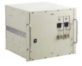
AD103 is an alarm announce system that provides local announce and local alarm through User station. It has a structure that ensures making announcements by selecting region within the ship through Alarm Announcement Stations, initiating and stopping certain selected alarms. With the management PC software, the whole system can be easily configured and fault conditions can be easily monitored.
