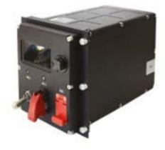
The Remote Control System has been designed to integrate into platforms without the need for software upgrades to the mission computer of the platform. The system can communicate directly with the electronic unit, thanks to the error-protected user interface for the firing operator and through RS422/CAN/Ethernet data channels. Its integral features make it a highly effective solution for integration programmes in terms of cost and time.
