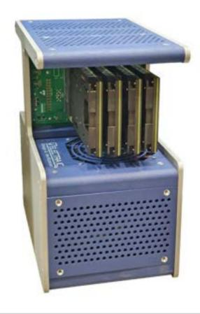
The VPX6-CH101 is a VPX open frame chassis designed for development and test. It supports custom or COTS backplanes up to 10 slots.
