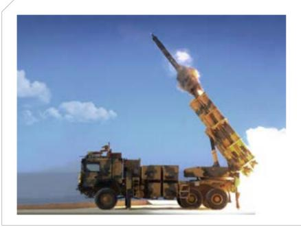
TRG-300 Guided Missile Missile provides accurate and effective fire power on high priority targets within the ranges 20 - 120 km. TRG-300 Guided Missile can be launched from ROKETSAN Multi Barrel Rocket Launcher [MBRL] Weapon System and other platforms with compatible interfaces.
