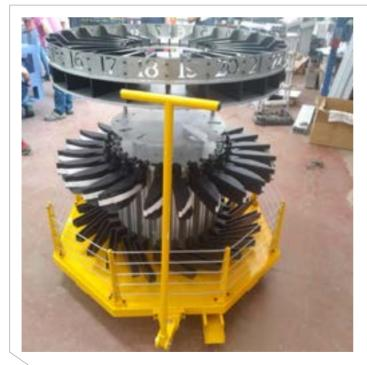
It is to safely store and transport fan blades and other critical components removed during CFM56-7B engine maintenance processes. This project is designed with a compact and durable structure to prevent part losses in workshop or field environments, save space, and accelerate maintenance procedures. Its ease of portability aims to enhance operational efficiency, providing both cost advantages and longterm support for safety and operational continuity.
