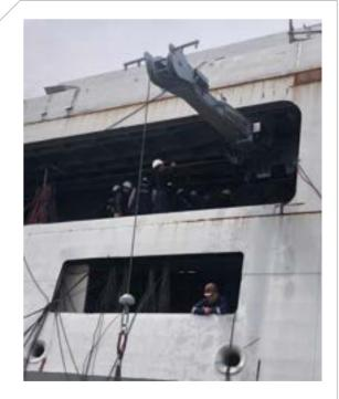
It will work as a part of the Ship and can be used for launching and retrieving the Boat from the sea.
