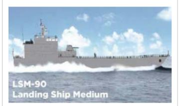
The LSM-90 is a Landing Ship Medium designed for transporting vehicles or troops ashore through the bow ramp by landing during amphibious operations. Additionally, in peacetime, it provides support for humanitarian assistance and evacuation/rescue operations.
