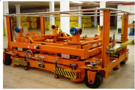
This Trolley is suitable for the installation and installation of degassed Main Landing Gear of A330 and A340 aircraft variants.
