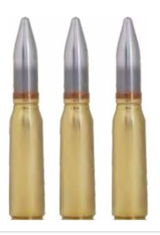
Has a maximum 168.02 mm cartridge length. The bullet material is Body (steel), Cover base (steel), Rotating Band (tombac) Fuse (aluminium). It has a M52 A3 B1 Electrical Primer. 20 mmx102 CARTRIDGE TP-T (M55 A2) has a maximum 168.02 mm cartridge length. The bullet material is Body (steel), Cover base (steel), Rotating Band (tombac) Fuse (aluminium). It has a M52 A3 B1 Electrical Primer.
