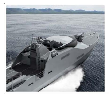
33m Guided Missile Fast Intervention Boats, were designed and built by DEARSAN according to the requirements of Turkmenistan Border Security Command. In 2014, the boats entered the inventory of Turkmenistan Border Security Command and have been operating effectively in the Caspian Sea since then.
