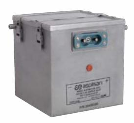
The battery is used in the C-130. It has a nominal voltage of 24 Volts, a nominal capacity of 27 Ah. It weighs 29 kg. The operating temperature range is -40°C to +71°C.
