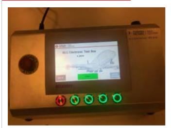
It performs the electrical and functional tests of the front landing gears of A320 and A330 aircraft.
