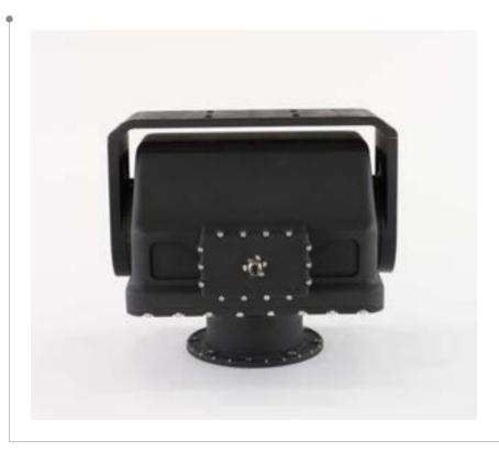
0510, one of our mini control and routing system models, is designed for reconnaissance, surveillance, antenna and optic fields. Our 0510 model, which weighs less than 5 kg, has a body dynamic that can support up to 15 Nm.
