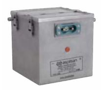
The battery is used in CASA CN-235. It has a nominal voltage of 24 Volts, a nominal capacity of 40 Ah. It weighs 36.5 kg. The operating temperature range is -40°C to +71°C.
