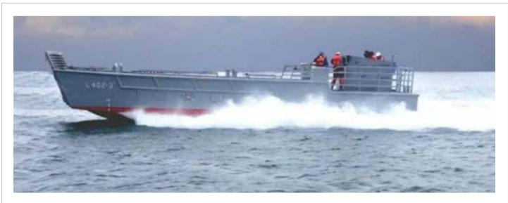
Built to conduct fast short range cargo& troops transfer between ship-shore, eight Landing Craft Vehicle and Personnel have been designed and constructed for Turkish Navy by ANADOLU Shipyard. They have been operational since 2017.
