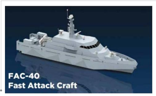
The FAC-40 is a Fast Attack Craft primarily designed for ASuW, as well as ISR and patrol missions, including the protection of oil platforms. With its weapons and systems, along with a maximum speed of over 35 knots, it is capable of conducting patrol duties, operations against asymmetric threats, preventing smuggling and piracy, safeguarding fishing and marine resources, and preventing illegal fishing.
