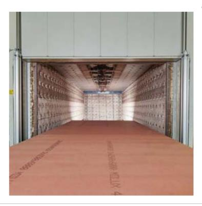
Miilux M690, highstrength structural steel supplied with minimum 690 MPa yield strength. M690 is preferred in areas with difficult load-bearing tasks.
