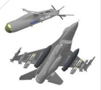
The TOLUN-IIR infrared seeker-guided munition features an integrated KKS/ANS/IIR guidance system for use against soft, moving ground targets. It can be dropped from the air platform via a multi-transport raft (SADAK-4T), and features a two-way communication mode and a man-in-the-loop firing mode.
