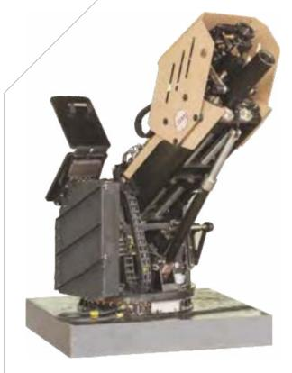
Has 120 mm caliber, is 1350 kg with an operational range of 9500m. It has 10 rds/min rate of fire and can be loaded either manually or semi-automatic.
