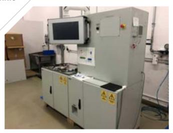
The bench developed for the testing of vacuum toilets in aircraft is capable of performing all electrical and functional tests.
