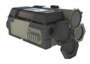
ENCEREK-M01 is a laser target designation unit designed for fire control units of land platforms. ENCEREK-M01 can operate at all Band I and Band II PRF codes defined in NATO STANAG 3733, hence is compatible with all NATO laser guided munitions with semi-active laser seekers, such as LGB's, Hellfire and Copperhead. The Unit can be controlled via serial interface and contains BIT function with high probability of error detection.
