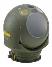
ASELFLIR-300T Electro-optical system is a reconnaissance, surveillance and targeting system which is designed for rotary wing platforms. The system contains 8-12 micrometer High Resolution Infrared Camera, DavTv. Laser Target Designator and Laser Range Finder.
