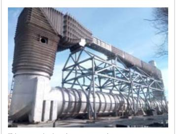
This system is aimed to carry out the necessary tests to ensure that the propeller systems of water vehicles operate quieter and faster and to reduce the physical damage caused to the propeller by the formation of steam bubbles.
