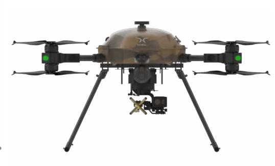
FALCON-DAD, also known as the Drone Hunter, is designed to effectively capture threat drone platforms using its integrated net gun payload as a Rotary-Wing Drone Hunter UAV system. It successfully neutralizes the threat drone using data from the integrated radar and imagery from the Electro-Optical and Infrared camera system.
