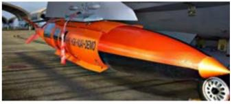
The Precision Guidance Kit (PUK) is a guidance kit that converts the existing 500lb Mk-82, 1000lb Mk-83 and 2000lb Mk-84 general purpose bombs into air-to-surface smart and precision strike capable ammunition with Global Positioning System and Inertial Navigation based guidance system. Designed by Tübitak SAGE, the Guidance Electronics Whole, Tail Whole and Front subassembly of the HGKs are produced by SDT A.Ş.
