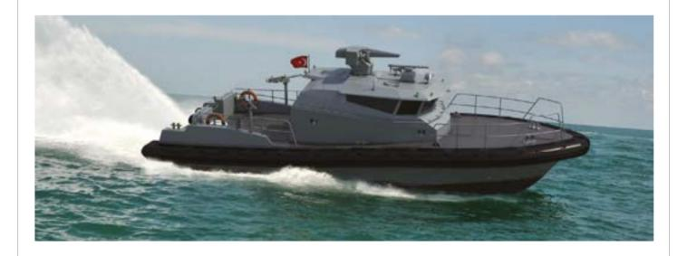
ARES 42 LC Fast Landing Craft is designed for various logistics purposes for carrying out a wide range of coastal and inland water transportation, fast personnel deployment duties, rescue and evacuation operations. Particularly designed and developed as a logistics support and landing vessel for naval and lawenforcement authorities in coastal and inland waters.
