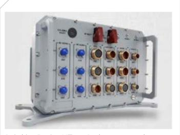
Switching Box is a Military Grade custom product designed by ElectralC. It performs Ethernet, RF, serial interface, power supply and discrete signal switching functionality to facilitate redundancy in radar systems.
