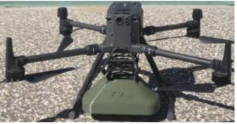
It is a new-generation Mine and IED detection system that GPR sensor developed with company's own resources has been mounted to a drone. It enables the detection of mines and IEDs under the ground surface by flying autonomously or manually up to 1 meter above the ground with the sensor, which is aproximately 2.5 kgs, integrated under drone. System, which has the ability of autonomous fly, can provide detection data to users by scanning a whole area in given coordinates.
