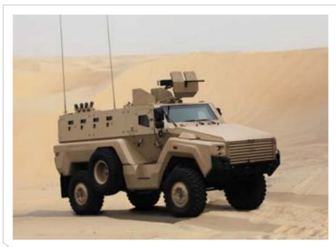
KAYA is specially designed and developed as a Mine Resistant Ambush Protected Personnel Carrier. KAYA provides enhanced mine and ballistic protection along with superior mobility in a wide range of demanding terrains under diverse climatic conditions. Single cabin monocoque body of KAYA carries up to ten troops including the driver and commander.
