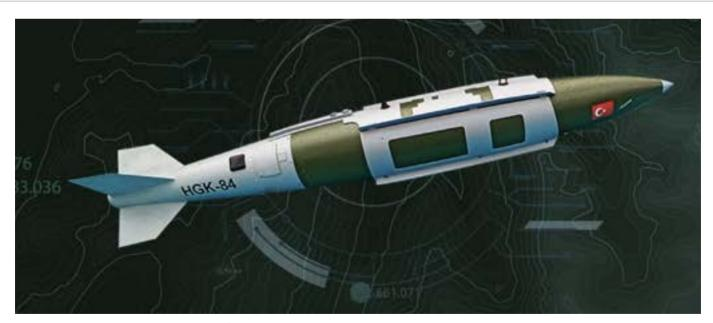
HGK-84 is a GPS/INS (GPS: Global Positioning System, INS: Inertial Navigation System) guidance kit that turns existing 2000 lb Mk-84 general purpose bombs and penetrator bombs into air to ground smart bombs.
