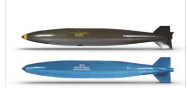
2000 lb. MK 84 GP AIRCRAFT BOMBs have two variants. MK84 HE is 884 kg, is 3797 mm long, has TNT as filler and the filler weight is 428 kg. MK84 PRACTICE is 884 kg, is 3797 mm long and it has Sorel Cement as filler.
