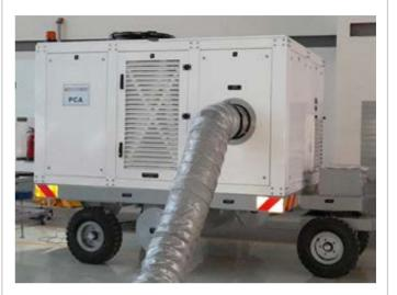
They are mobile systems that provide energy and conditioned air needs for structures such as tents, hangars, and warehouses.
