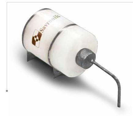
ARK-101 is a hermetic, pressurisedgas, three-electrode high voltage triggered arc switch consisting of ceramic-metal parts. It ensures that the pyrotechnic elements remain safe after the installation of high voltage capacitor in electronic plugs.
