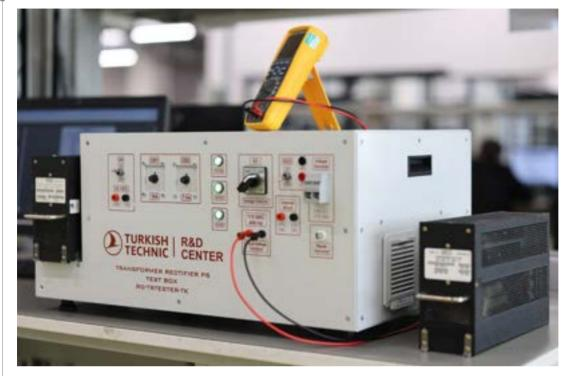
This is a test bench that will be used during the electrical maintenance and testing of the 'Transformer Rectifier Power Supply' component found in B373 aircraft.
