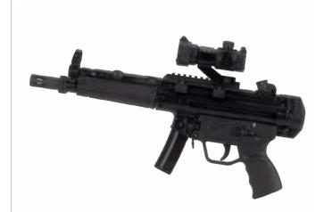
Has Roller-Lock Delayed Blowback Action. It has 10/15/30 magazine capacity and is 2500 g. Effective range is 100 m.
