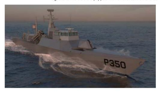
controlled naval weapon systems to provide versatile firepower that can be adapted to a wide variety of potential scenarios. The vessel has a suite of naval communications equipment, combat management system, electro-optic (E/O) sensors and 3D Naval Radar.
