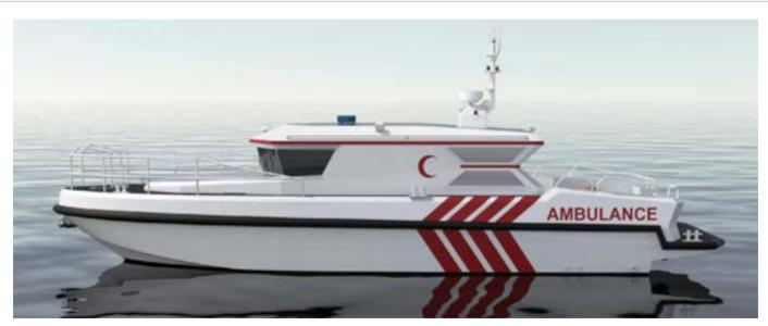
ARES 44 AMBULANCE is inspired from an innovative hull design of special OP's support craft. Iterative elaboration has been applied to the underwater body, resulting in low resistance and good seakeeping hull form, combined with excellent navigation capabilities. ARES 44 AMBULANCE has been designed for rapid ambulance response, patient and casualty transfer operations, incident response and SAR operations.
