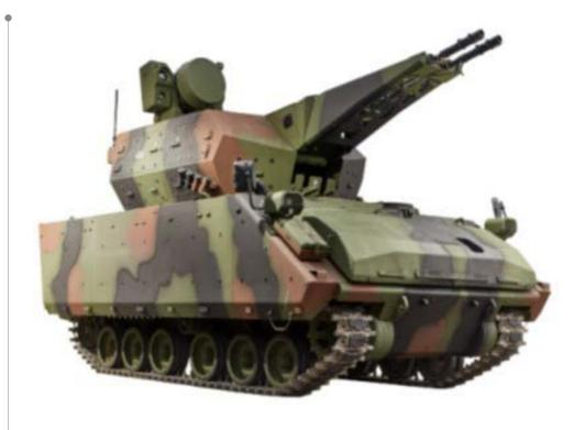
The KORKUT system is an air defense system developed by ASELSAN in order to effectively carry out air defense of mobile elements and mechanized units. FZK manufactures the armored gun towel body of the KORKUT air defense system.
