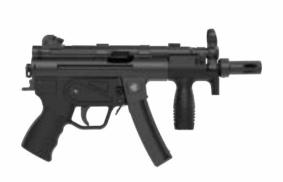
Has Roller-Lock Delayed Blowback Action. It has 10/15/30 magazine capacity and is 2090 g. Effective range is 100 m.
