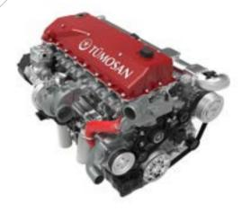
It is Tümosan's 7.8-liter inline 6-cylinder, water-cooled industrial engine. This engine, which has a turbocharger aspiration and common rail injection system, produces 336 kW nominal power at 2400 rpm and provides 1600 Nm of torque between 1300-1900 rpm. The high-performance TMSN X7.4 motor stands out for its low fuel consumption and is a reliable choice for military and industrial applications.
