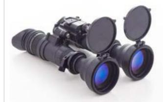
NOVA A510 Night Vision Binoculars are night vision systems working on image intensifier technology. The googles provide superior image even at low light conditions such as starlight illumination. With A510, users obtain image with low halo effect and high resolution. The auto-gating feature of the tubes gives users the ability to operate even on bright light sources such as city lights.
