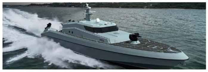
ARES 34 CB is a proven design developed for transport of offshore support personnel, deck cargo, below deck cargo such as fuel and potable water to and from offshore installations. It is designed with advanced seakeeping characteristics. ARES 34 CB has been designed and built for a Private Oil Company.
