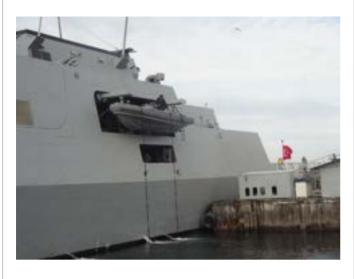
It is a system designed to take the boat from the location on the ship to the sea and/or to take it from the sea to the location designed for the vehicle on the ship.
