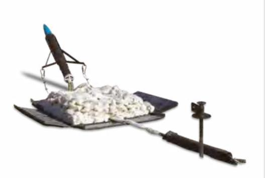
Can clear pressure and single impulse type mines (TM-45, TM-57, TMKR-2, MK-56 and similar mines). Total weight of the system is 2800 kg (Included trailer, launcher, line charge and rocket group). It uses 400 kg C-4 as explosive and 2.75" G1 Rocket. The flight range is 200 m and it has a shelf life of 10 years.
