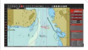
It has been developed to train operators who will work in Vessel Traffic Services (VTS) systems. The simulator allows operators to learn the concepts needed for planning vessel traffic through the software. It can be integrated with FMBS and Marine Pollution Simulators.
