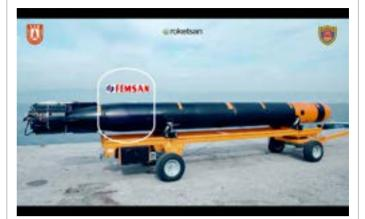
Femsan has developed and continues to produce the main propulsion unit (Electric Motor, Driver, and Control Card) of Akya. Akya stands out as one of the national torpedo systems of the Turkish Navy, operating effectively thanks to these critical components manufactured by Femsan.
