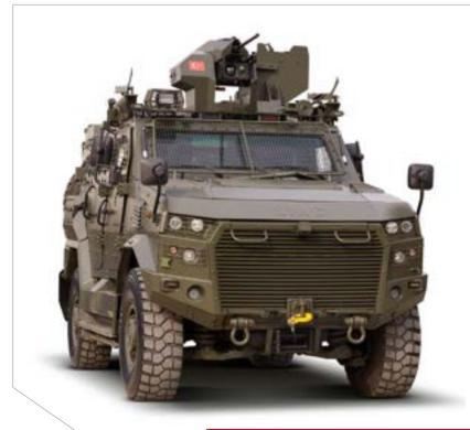
AMAZON 4×4 MPAV (Multi Purpose Armored Vehicle) which can carry up to 7 personnel is the lightest member of our Armored Vehicle Family weighing only 14.5 Tons. It provides a high protection level according to NATO STANAG 4569 Standards against both ballistic and mine threats.
