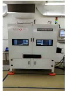
It is used to perform the "overspeed" procedure after the repair/ maintenance of IDG rotors.
