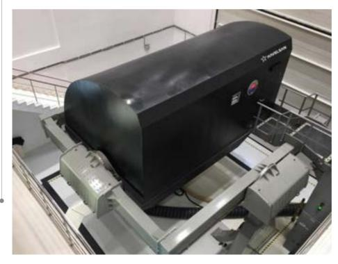
Submarine Diving Simulator which simulates T.C. U209 PREVEZE / GÜR class submarines in the inventory of the Naval Forces Command, have been designed and manufactured in order to complete the preparatory and periodic training of diving cabin crew without using the submarine.
