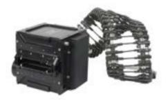
Booster Mechanism allows the gun to load 12.7x99mm NATO ammunition from bullet belt from a 3 meter distance. Booster Mechanism allows the gun to load bullets when chain wheels in the mechanism is triggered by motor, since the power of the gun is not enough to load all kinds of bullets from a 3 meter distance.
