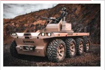
KAPGAN is an Autonomous Heavy Class UGV designed to accompany troops in different missions with its high maneuverability, especially in harsh environmental conditions. In addition to cutting edge payload options for different functions such as the Upgradable Perimeter Surveillance System, the integrated 30 mm Gun with an effective range of 2 km provides high deterrence at low volume with its armor-piercing feature against land and air targets in the field.
