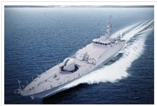
57m Tuzla Class Patrol Vessels were designed by Dearsan according to the requirements of the Turkish Naval Forces Command and a total of 16 were built. Inventoried in 2010, Tuzla Class Patrol Vessels perform all assigned missions effectively in the Black Sea, Marmara, Aegean and Mediterranean seas.
