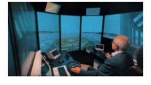
This simulator is based on the MARSIM-FMBS platform and is designed to provide training for Tug Masters. In our DNV-certified simulator, training is available with three different types of tugboats: Voith Schneider, Azimuth Propeller, and Standard Tug. The simulator is designed with screens that can create a 360-degree 3D scene. Various training areas can be added to the simulator, enabling more realistic training scenarios.
