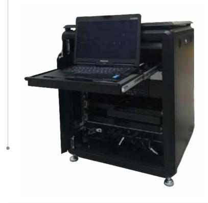
Savronik's interoperatiliy system (Savrolink) is a gateway structure that establishes a bridge which provides voice and data transfer capabilities between HF, VHF, UHF radios, line-of-sight and beyond line-of-sight datalinks, mesh systems and IP based devices (IP telephones etc.) that operates different frequency bands, waveform and technologies.
