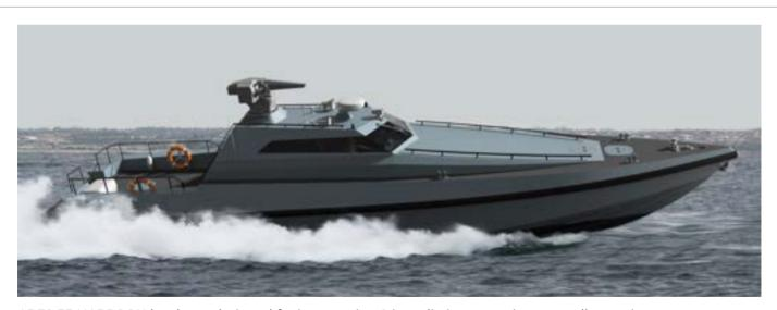
ARES 55 HARPOON has been designed for interception & interdiction operations, as well as antismuggling, SOF insertion and extraction, surveillance and patrolling missions. The craft is equipped with an auto-stabilized remote-controlled naval weapon system to provide versatile firepower that can be adapted to a wide variety of potential scenarios. The vessel has a suite of naval communications equipment, electro-optic (E/O) sensors and X-Band Naval Radar.
