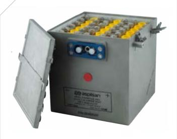
The battery is used in CASA CN-235. It has a nominal voltage of 24 Volts, a nominal capacity of 40 Ah. It weighs 36.5 kg. The operating temperature range is -40 $^{\circ}$ C to +71 $^{\circ}$ C.
