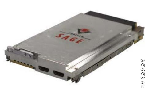
Signal Processing Board OpenVPX (ANSI/VITA 65) 3U format, compatible with OpenVPX standard, based on System On Chip (SoC) Single Board Computer. It is designed for signal processing needs.
