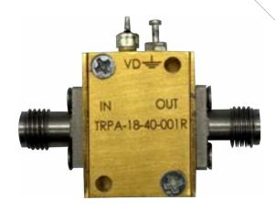
TRPA-18-40-001R is a compact microwave RF amplifier with connectors. Operating within a frequency range of 18-40 GHz, the amplifier is equipped with 1 RF input and 1 RF output, providing high gain and low in-band ripple. It offers low noise and return loss across a broad frequency range. The unit does not require a negative bias voltage and is powered from a single source. It is an effective and ideal choice for applications needing reliable signal amplification at high frequencies.
