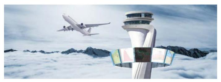
OpsEye is a traffic tracking system for the apron area that supports flight operation control units and directly contributes to the decision support mechanism in tactical operation. The system provides instant information about airplanes such as door closing, push-back, airborne, approaching and live monitoring of ground traffic, and location identification. It operates in integration with the airline's internal operational systems.
