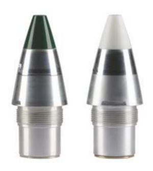
The Electronic Time Fuzes has two variants: MKE MOD 124 and MKE MOD 134. MKE MOD 124 function is Electronic time, PD Mode. It has a weight of 700 g, has a booster explosive of approximately 5 g Black Powder and it is used in Spin-Stabilized HE Ammunition between 105-203 mm. MKE MOD 134 function is Electronic time, PD Mode. It has a weight of 685 g, has a booster explosive of approximately 22 g RDX/Tetryl and it is used in Spin-Stabilized Smoke/Illumination Ammunition between 105-203 mm.
