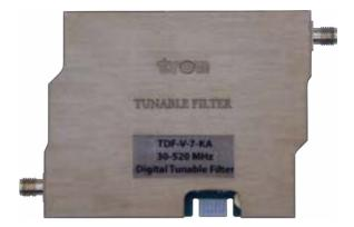
The TDF-V-7-KA Digital Tunable Filter, which can be used in both transmit and receive situations, is a bandpass filter that adapts to changing frequency values. By shifting the centre frequency, it aims to reduce interaction with ambient electromagnetic conditions and to provide band cleaning by suppressing signals at other frequencies.
