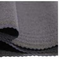
Protective filters produced from spherical activated carbons with high surface area and large pore structure are used in CBRN protective suits. It is light, flexible and has high protection value.
