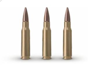
Has a 71.12 mm cartridge length. The bullet material is Gilding Metal, Lead Core (Lead-Antimony Alloyed). It has a 7.62 mm Primer, Boxer.
