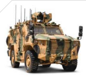
VURAN 4×4 MPAV (Multi Purpose Armored Vehicle) can carry up to 9 personnel and provides a high protection level according to NATO STANAG 4569 Standards against both ballistic and mine threats. Roles & Variants: Troop Carrier - Combat Tactical Vehicle - Mortar Launcher Vehicle - Multi-Rocket Launcher Vehicle -Laser-Guided Missile Launcher Vehicle
